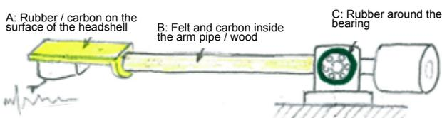
Fig 6: Series damper structure
