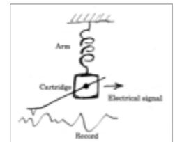
Fig 2 (A) Conceptual diagram of signal loss and sound distortion due to vibration of the arm
