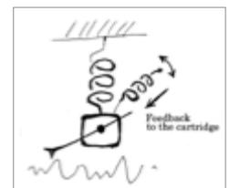
Fig 2 (B) Conceptual diagram of signal loss and sound distortion due to vibration of the arm
